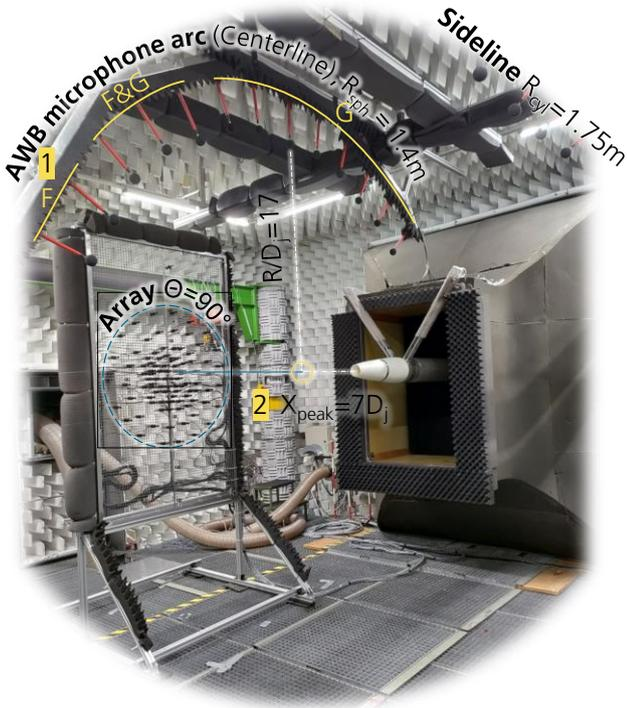
**Figure 1:** Static jet noise test setup for validation of the dual stream engine models at AWB, July 2024. Instrumentation is setup as a close listener  $R_{\text{mic}}/D_j = 17 \dots 50$ .
