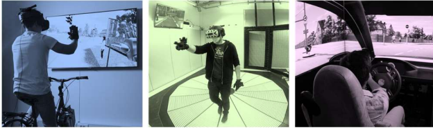
Figure 3: MoSAIC laboratory human-in-the-loop simulators: left cyclist, center pedestrian (Omnideck), right driver
