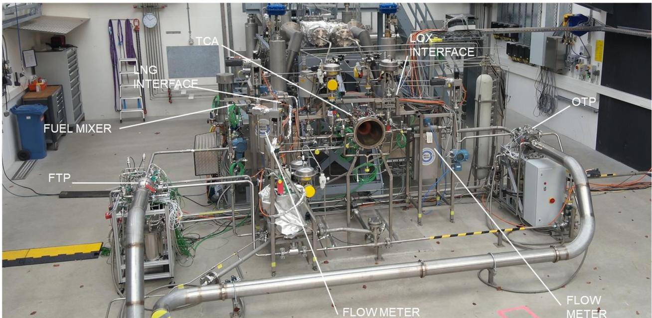
Fig. 3. LUMEN layout at test bench P8.3
