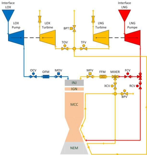
Fig. 1 Schematic representation of the LUMEN demonstrator architecture.
