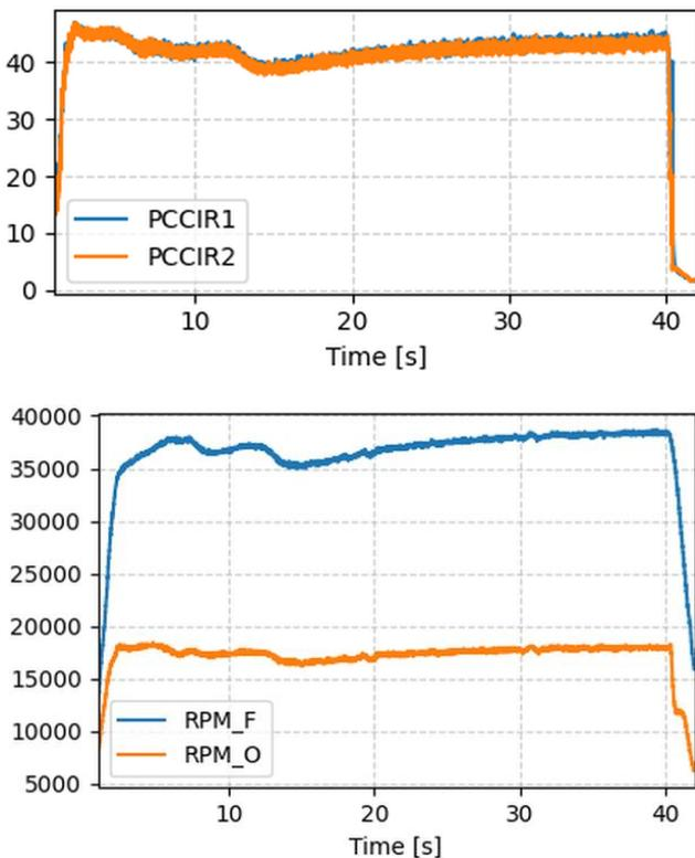
Fig. 5: combustor pressure  $P_{cc}$  and rotational speeds of the TP in the second test run
