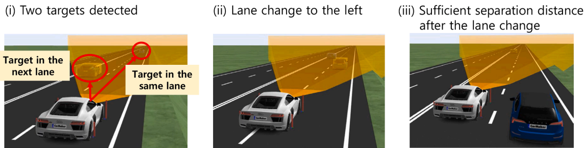
Fig. 14. Simulation scenario performed with the Carmaker simulator [17], where two target vehicles are detected.
