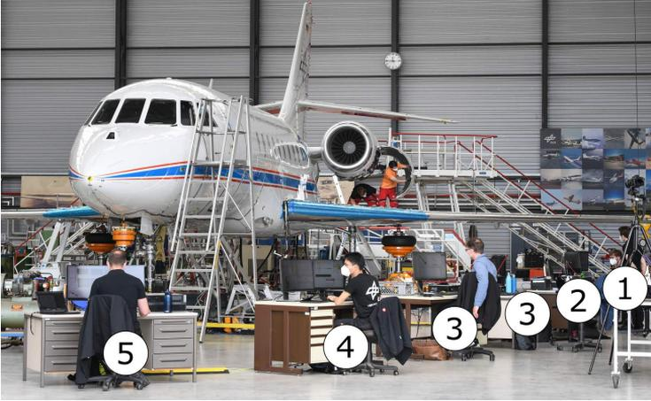
Figure 4.4: ISTAR in GVT with manual analysis chain (1-4) and SAGVT (5)
