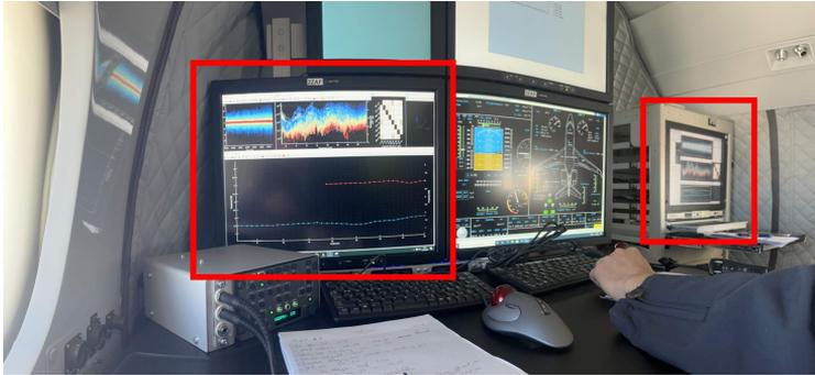
Figure 5.6: Analysis computers with real-time modal parameter monitoring system in ISTAR FVT
