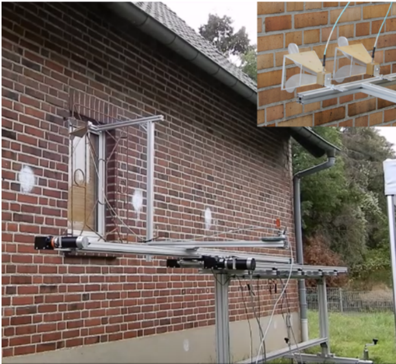
Figure 3.11.: Rack with movable antennas for microwave radar scans of the interior structure of an exemplary case study building wall [9].
