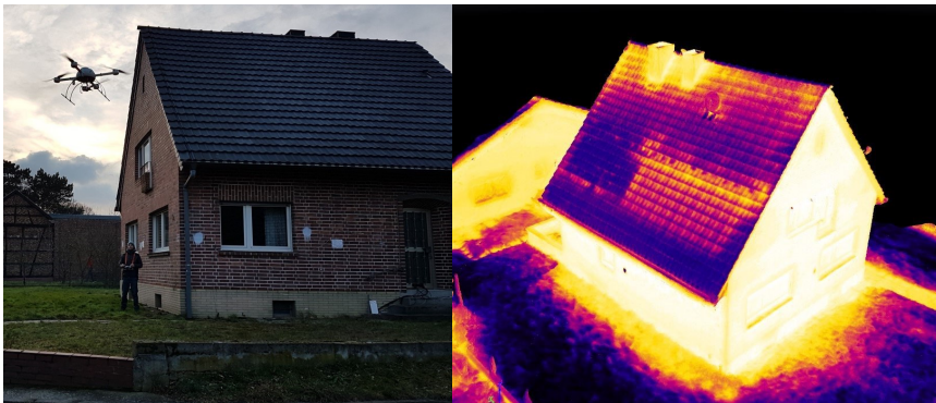
Figure 3.10.: IR image acquisition from UAV on a winter early morning (left) and point cloud of the case study building (of Figure 3.9) textured from the results using Pix4D Mapper (right) [9].
