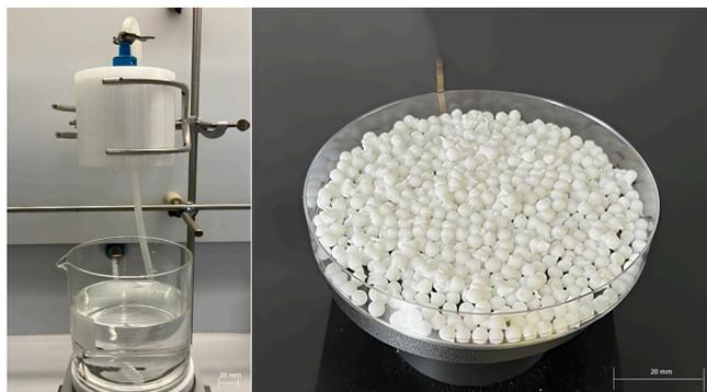
**Figure 1.** Illustrating the conventional multinozzle dropping setup (left) and aerogel beads (right).
