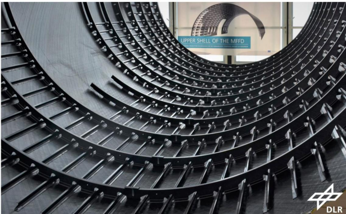
**Fig. 5** Stiffened shell structure on the Multifunctional Fuselage Demonstrator (MFFD), according to [5]
