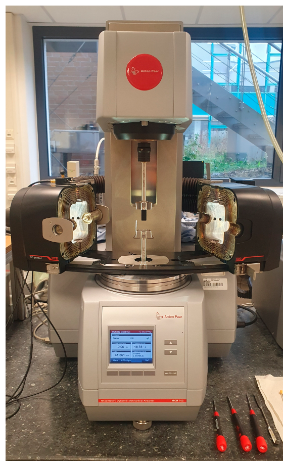
Figure 3. Rheometer Anton Paar MCR 702 with test specimen.
