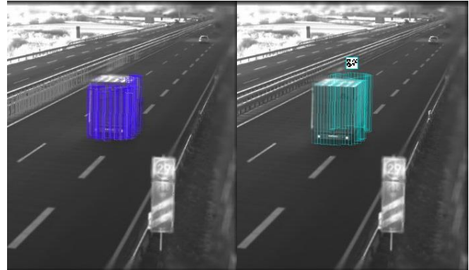
Fig. 4: Object detection. Accumulation of voxels (blue) in the left image, which form a bounding box (turquoise) in the right image.
