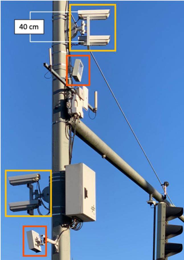
Fig. 3: Multi-sensor system on the pole: The upper system is directed outward, while the lower system faces the intersection.
