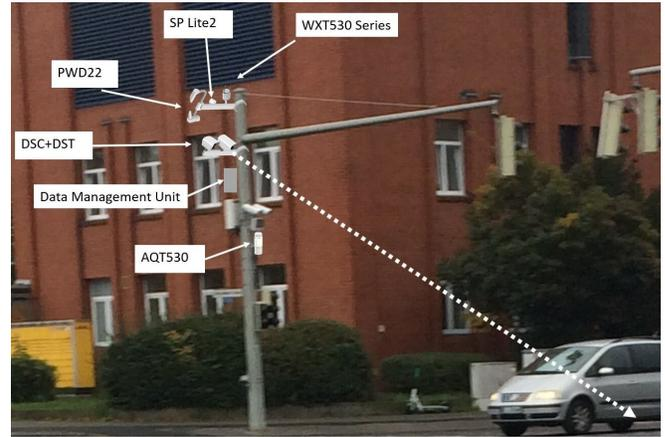
Fig. 4: Weather station mounted on the pole, including sensor labels and the measurement range of the DSC and DST sensors (dashed lines).
