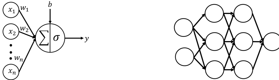
Figure 2.7: Schematic figures of artificial neural network neuron (left), connected artificial neural network (right)
