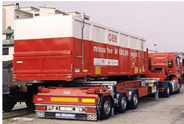
Figure 23: Horizontal handling of a Mobiler container from a truck to a waggon in parallel position. Source: Rail Cargo Group, ÖBB, Public Domain, 1995
