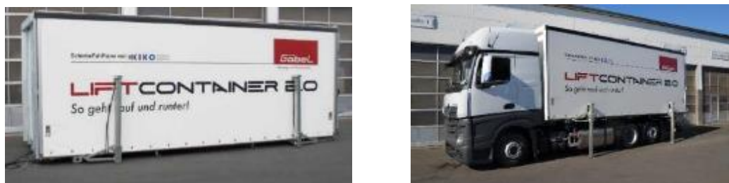
Figure 38: Liftcontainer with folded legs and, secondly, with extended legs prepared to be docked on to a truck. Source: ©Liftcontainer.de, 2020
