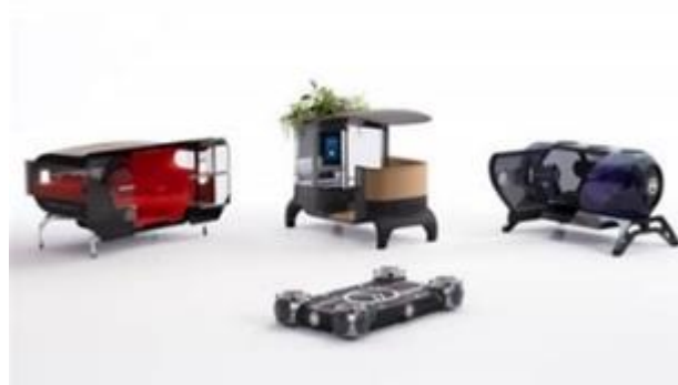
Figure 13: Citroën Skate round-wheel carrier and its three transport units Sofitel En Voyage, Citroën X JCDcaux, and Citroën X Accor. Source: ©Citroën, 2023
