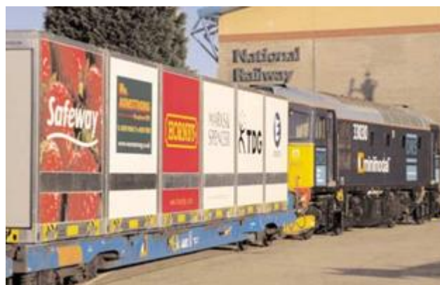
Figure 5: Minimodal freight system of Rail Freight Limited shown for the first time at the National Railway Museum in York in September 2002. Source: Railwatch, Public Domain, 2002
