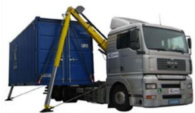
Figure 30: Sidelifter in operation. Source: BoxMover, Public Domain, 2010
