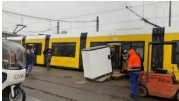
Figure 47: A cargo-bike container is transhipped onto a tram at the BVG's Berlin Lichtenberg tram depot. Source: ©ONOMOTION, 2021
