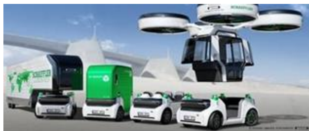
Figure 15: Visualisation of Schaeffler's modular concept with different cargo transport units, a passenger version of the rolling chassis and the drone variant. Source: ©Poschwatta, 2018
