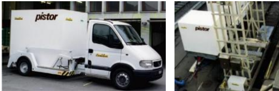
Figure 37: Combibox carried by an adapted van and being transhipped on to a freight waggon. Source: Tiefbauamt der Stadt Zürich, Public Domain, 2002
