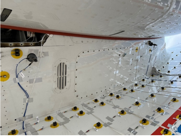
Figure 2: Two fixed TVA position at the bottom of the pylon, airplane front is left in picture
