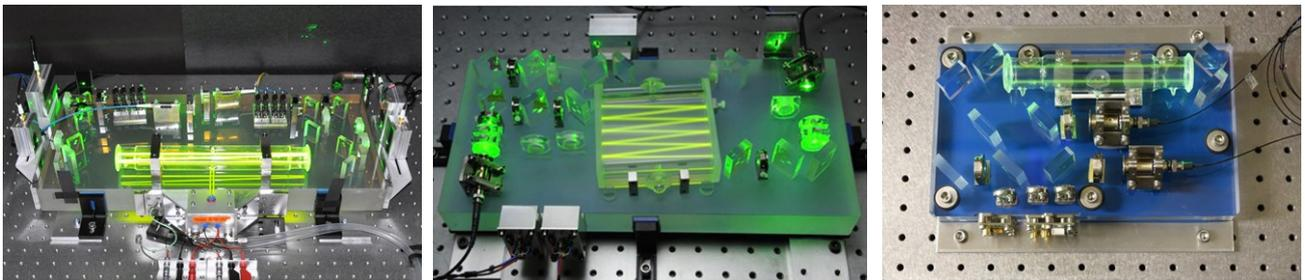
Figure 2. Photographs of realised iodine spectroscopy units at DLR QT
