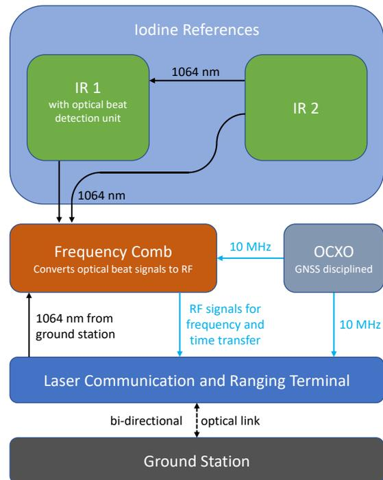
Figure 3. Block diagram of the COMPASSO architecture [10]. The two iodine references (IR 1 and IR 2) can be compared to each other with the included beat detection unit. With the frequency comb the optical frequency can be transferred to the RF domain and compared to an GNSS disciplined OCXO or stabilised laser which is transferred with a bi-directional optical link between the LCRT and the ground station.
