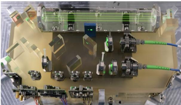
Figure 6. Photograph of the COMPASSO iodine reference spectroscopy board from DLR QT [10]
