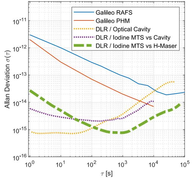
Figure 1. Comparison of current GNSS microwave clocks with optical clock technologies from DLR QT. The currently on Galileo deployed microwave clocks (solid lines) reach from  $>10^{-12}$  at 1 s integration time to  $>10^{-14}$  at 1000 s integration time. The DLR optical frequency references (dashed lines) have instabilities in the low  $10^{-15}$  range.
