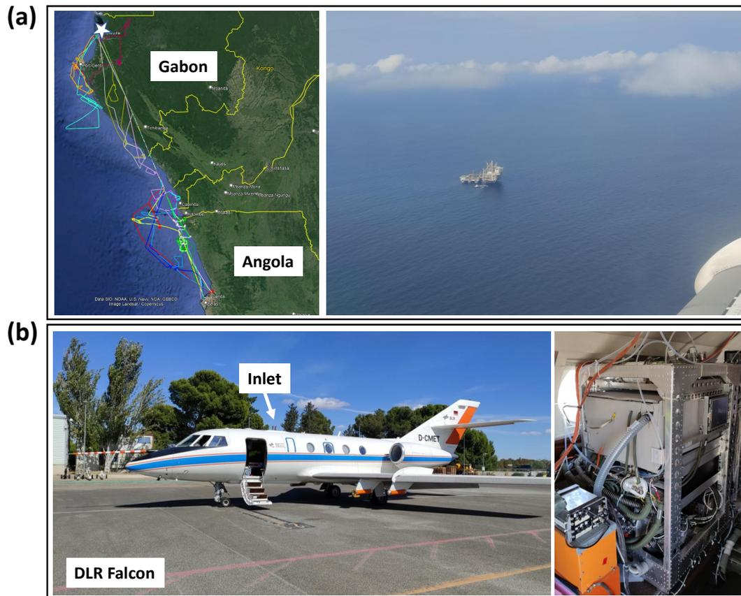
Figure 5.7: (a) Flight tracks of the 15 MTGA flights off the coasts of Gabon and Angola. A photograph of an oil platform as seen from the research aircraft is shown on the right. (b) Photograph of the DLR Falcon (Dassault Falcon 20 E-5) research aircraft on the left and the DLR-QCLS mounted inside the cabin on the right side.
