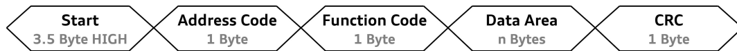
Figure 13.4: Structure of the Modbus RTU protocol for controlling the DC-DC converter DPS5015 [525].
