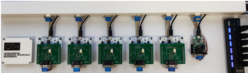
Figure 5.17: Hardware test setup consisting of five nodes, which consist of a custom CAN-FD-PHY-board and an ARM-Cortex-M4 based microcontroller [304]
