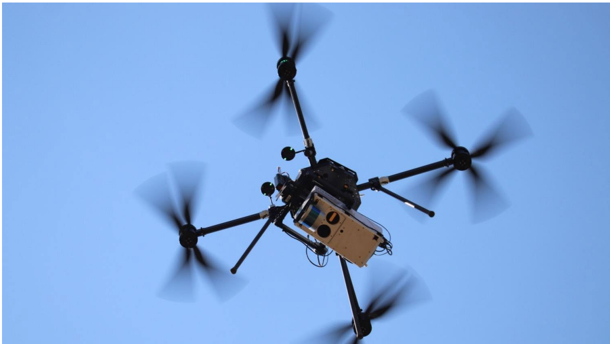
Figure 1 HySpex hyperspectral imager mounted on a drone platform.
