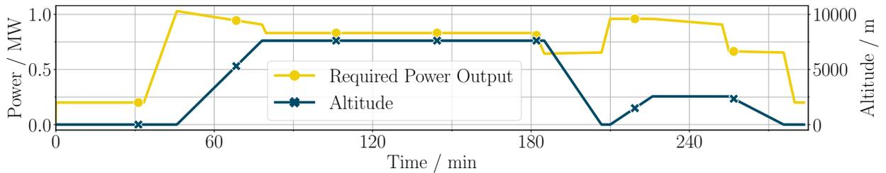
**Fig. 2 Turboprop mission definition consisting of the altitude and the required power output.**
