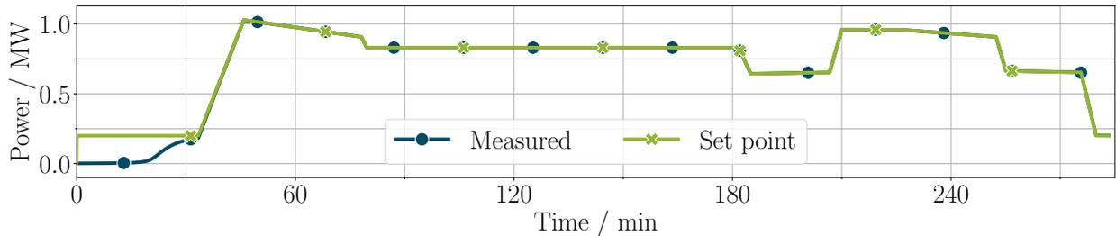
**Fig. 5 Analysis of the control of the electric power output of the fuel cell stack over the mission time with.**
