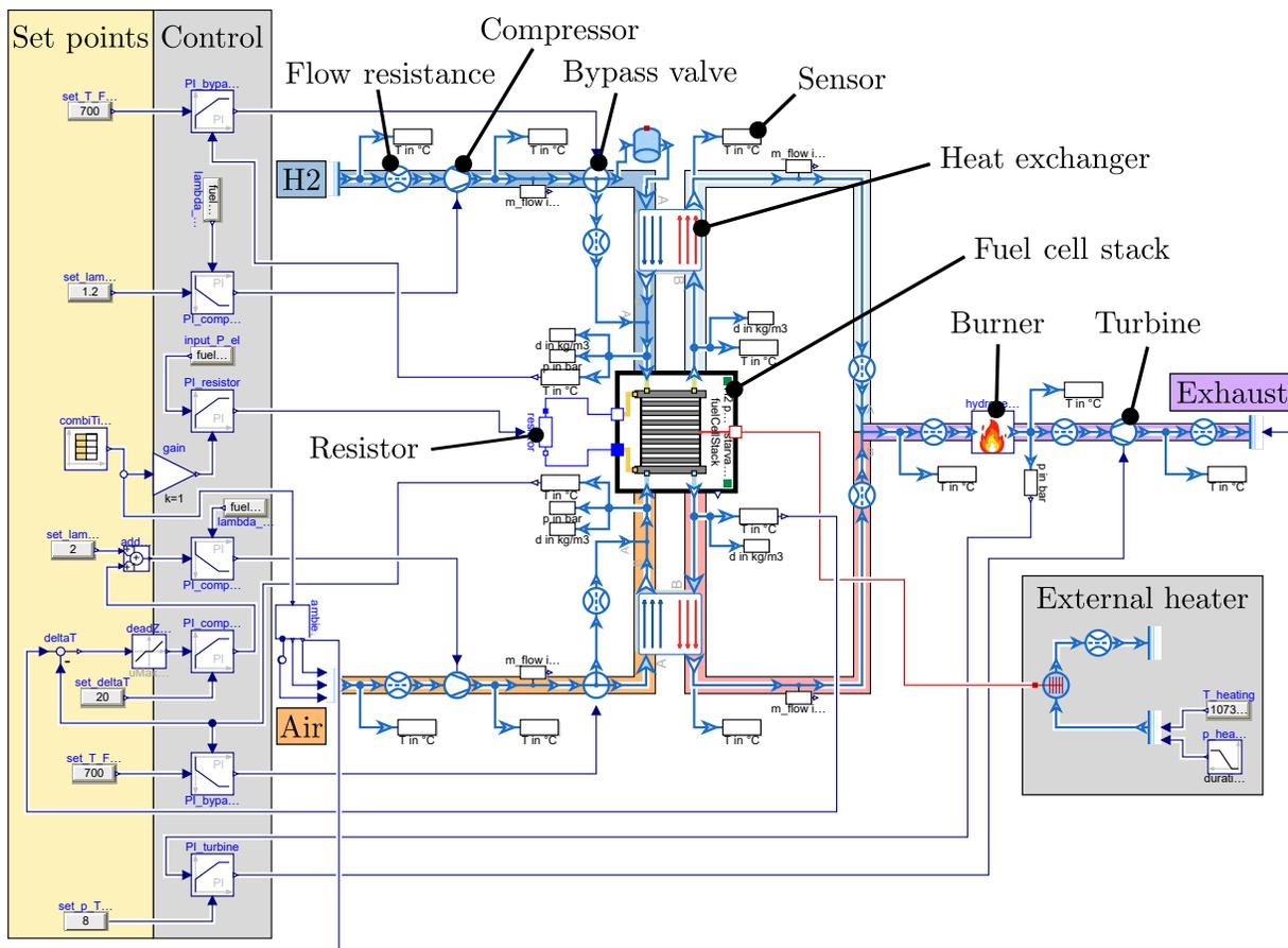
Fig. 1 Simulation setup of the fuel cell system and its control scheme in Modelica.
