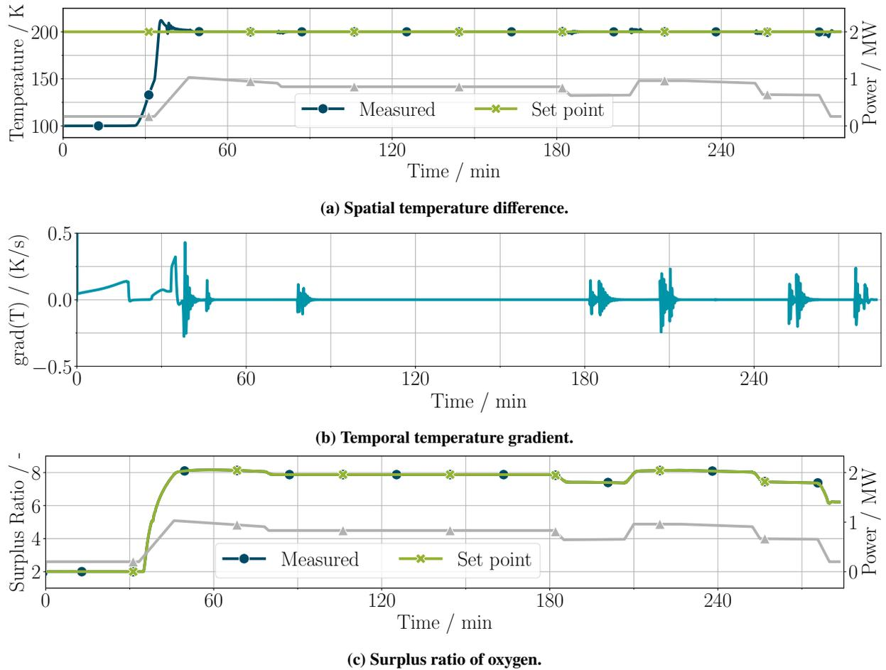
**Fig. 7** Analysis of the cascaded control of the air compressor with the spatial temperature difference in (a), the temporal temperature gradient of the average fuel cell temperature in (b) and the surplus ratio of oxygen at the cathode inlet in (c).
