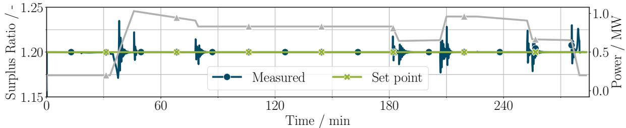
**Fig. 3 Analysis of the control of the hydrogen surplus ratio over the mission time; the required power output is shown in grey as orientation.**
