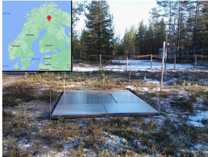
Fig. 7. Snow scale that measures the SWE of the snow pack at the IOA [31] with location on the map. The accumulated snow is weighted over the center plate.
