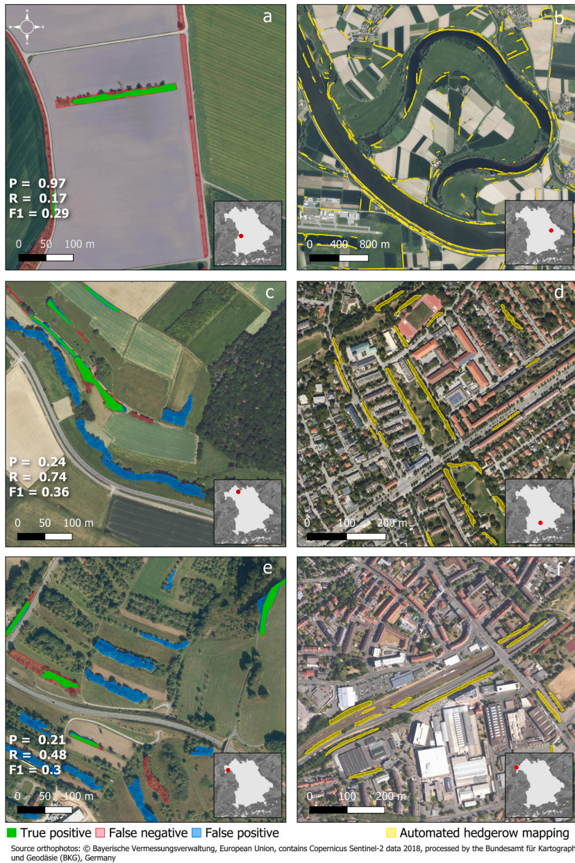
Fig. 8. Typical error types in the automated hedgerow mapping within the test regions with the original orthophotos at 20 cm resolution. True positives are displayed in green, false negatives in red and false positives in blue. The precision (P), recall (R) and F1-Score (F1) were calculated for the areas visible in each subset. Example a) shows undetected hedgerows located in the district of Dillingen. In c), Hassberge, riparian vegetation is erroneously detected by the model and e), Miltenberg, shows misclassifications due to complex cultivation patterns. Other errors found in the Bavaria-wide mapping are the classification of b) riparian vegetation in Straubing, tree rows along alleys and green urban space classified as hedgerows in d) Munich and f) vegetation along railways in Aschaffenburg.
