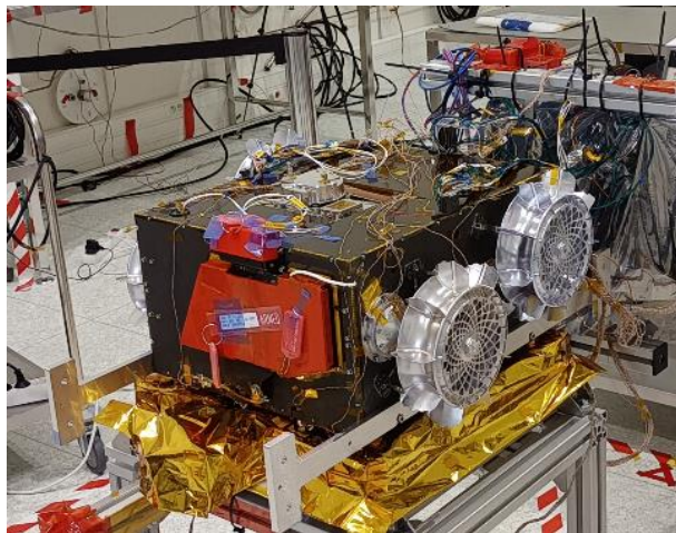
Fig. 3. IDEFIX flight model (FM) during tests at CNES. Note that solar generator is not integrated in this configuration. (image: CNES)
