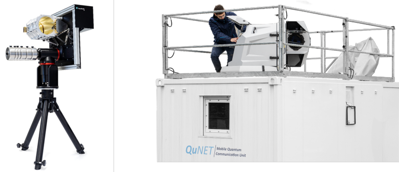
Figure 2. Left: Transportable FSO terminal 1 (TFT-1) mounted on a motorized telescope tripod. Right: QuBUS with periscope assembly on its roof (cf. Sec. 3.1.3).
