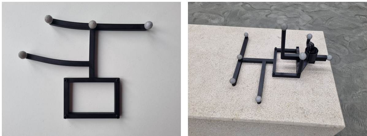
Figure 5.6: On the left, the effect of extended sunlight exposure on the Base Marker, bending the Polylactic Acid (PLA) beams and rendering the target unusable. On the right, the setup of the test conducted to measure the real position of the end-effector reference frame with respect to the one of the Base target.
