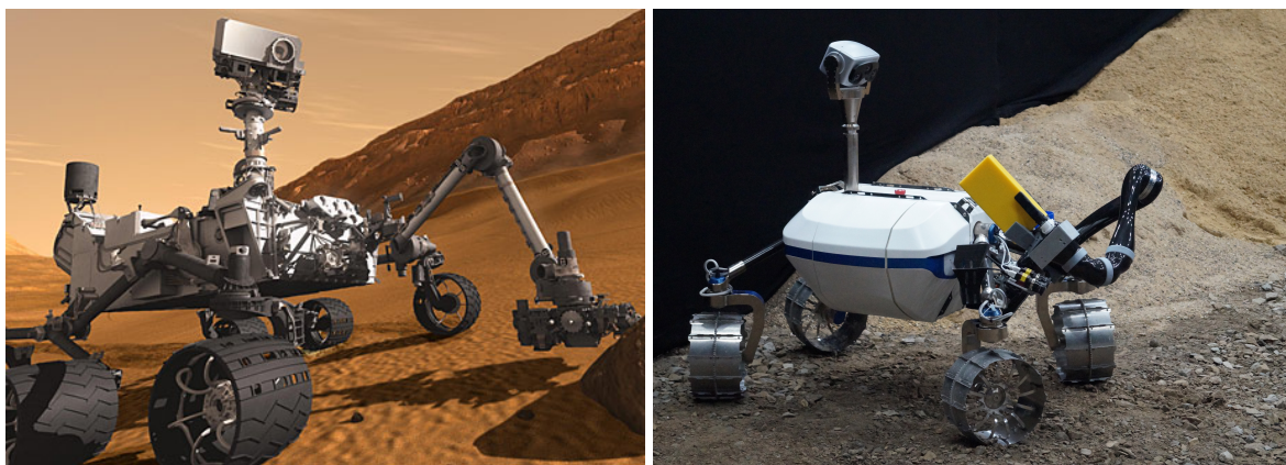
Figure 1.1: On the left, NASA's Mars Curiosity Rover and its advanced manipulator "The Arm" (NASA, 2024). On the right DLR's Lightweight Rover Unit (LRU) while operating its extremely dextrous robotic arm (Wedler et al., 2015).
