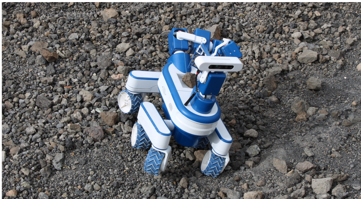
Figure 8.1: The Lunar Rover Mini navigating the rough terrain of Vulcano, in a precarious situation close to tipping over. In this scenario, utilizing the arm to shift the center of mass of the rover or leveraging it against the terrain could aid in recovering the rover to an upright position.
