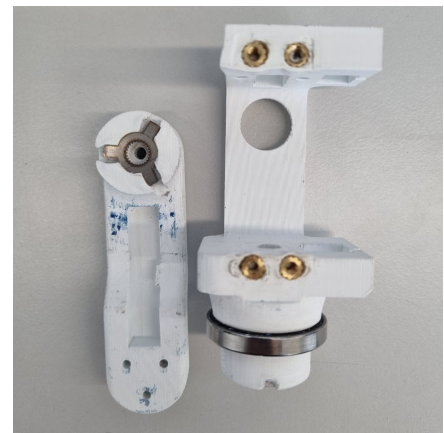
Figure 5.8: Picture of the components affected by the meltdown of one of the servos during the first test runs. On the left, it is clear how the melting ASA allowed the inserts to slip out of the reserved holes and the damage at the base of the servo's wiring. On the right, the damage to the other component is more clear, with the huts designed for the servo metallic heads fatally worn out.
