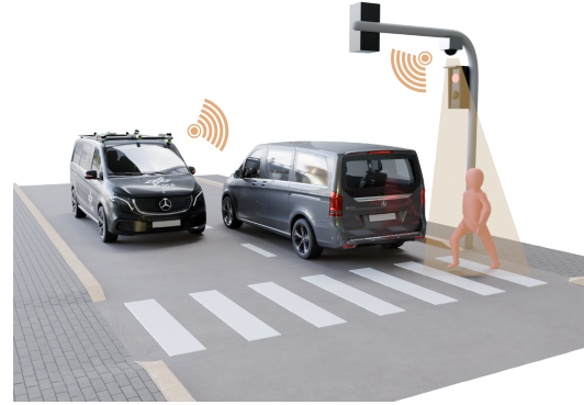
Figure 6: Example of the advantages when combining infrastructure and local autonomous driving, the CAV is driving along a road, and unable to see the person running towards it, as they are hidden behind another vehicle.
