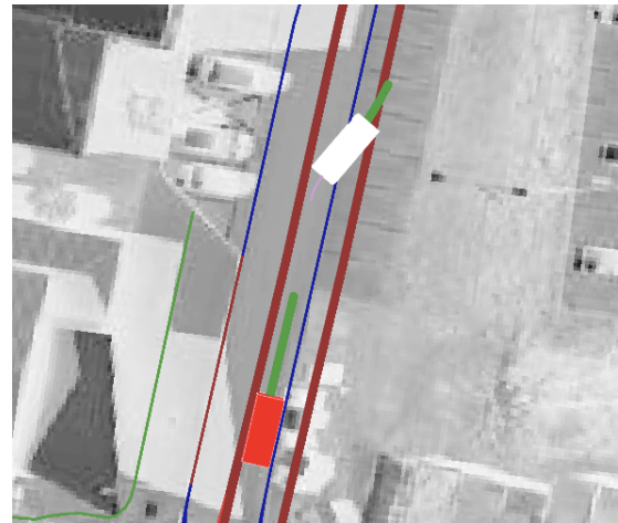
Figure 12: Ego Vehicle (white) leaving the safety corridor to form emergency lane for emergency vehicle (red) to pass by.
