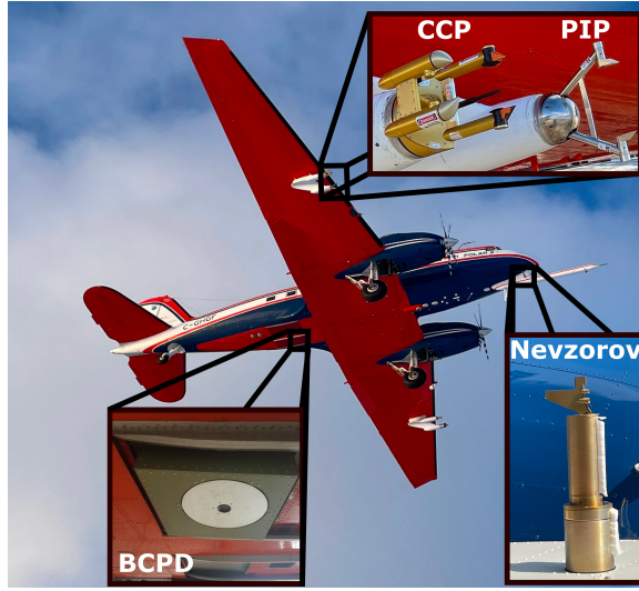
Figure 5.2: : Installation locations of the DLR instruments during the HALO-AC 3 campaign. The BCPD was located in the fuselage behind a roller-door system that was opened during the flight.
