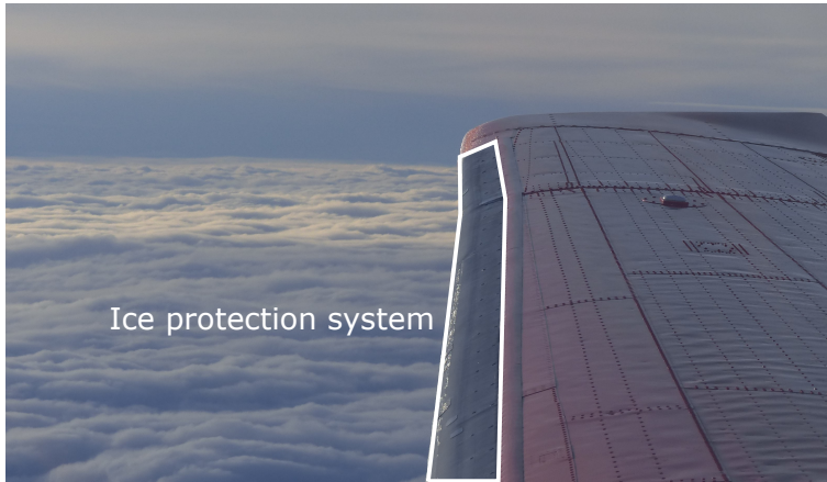
Figure 1.1: Ice protection system on the wing of the Polar-6 aircraft of Alfred-Wegener Institute. Image courtesy of Christof Lüpkes.
