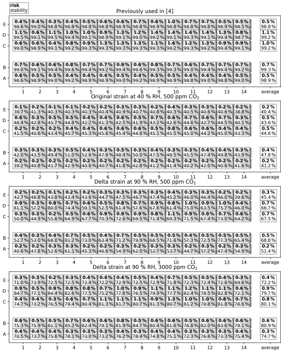
Fig. 1 Infection risk written in bold and virus stability averaged over 70 possible seat locations of the index person on all seats for four different inactivation rates. Seat column averages are shown on the right hand side
