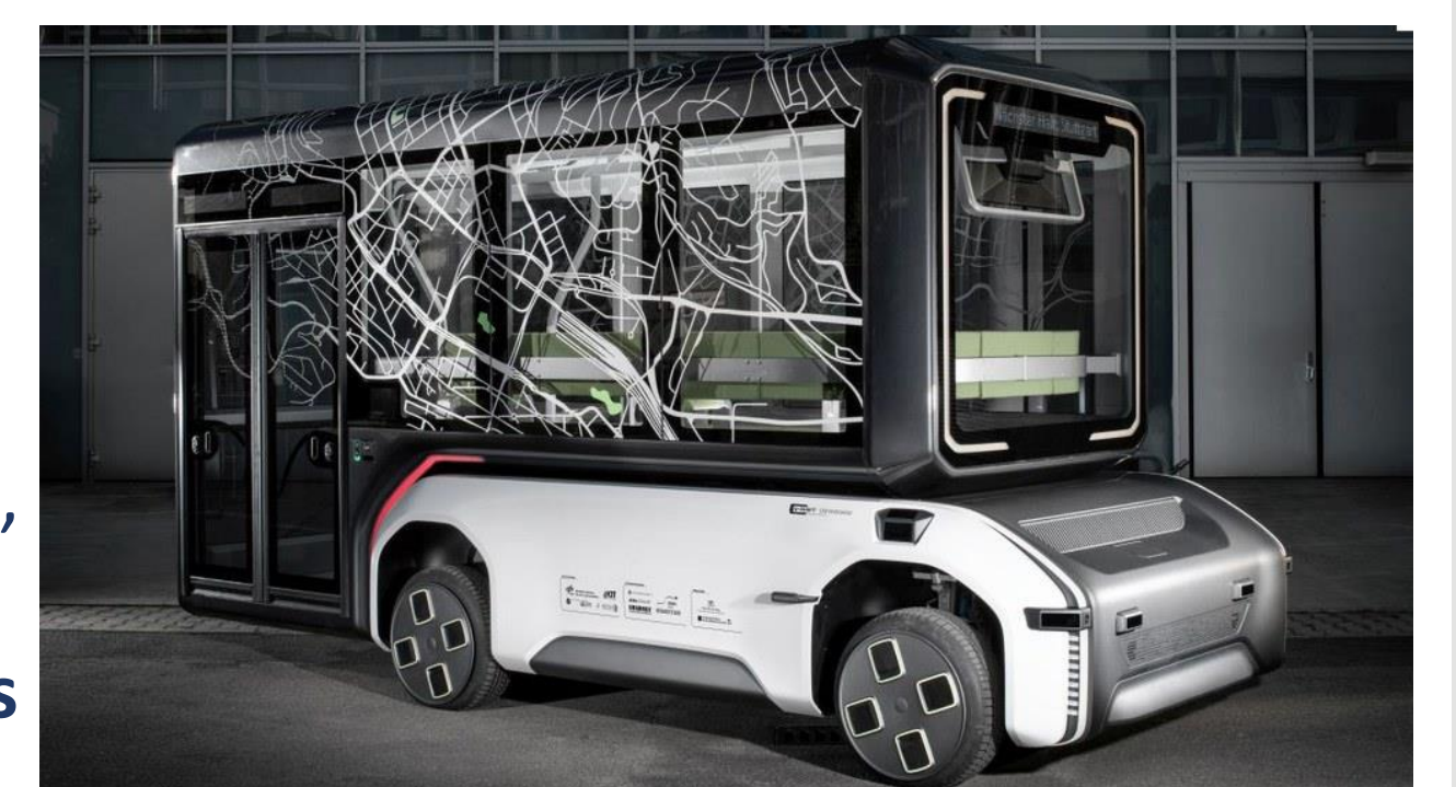
The U-Shift with the driving module and the interchangeable passenger capsule
