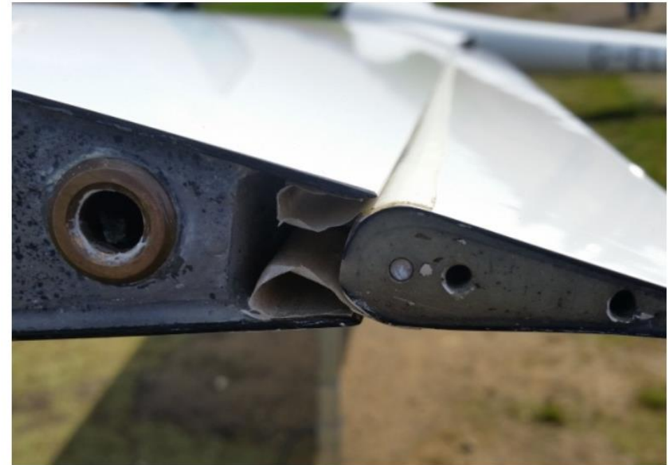
Aileron seal of the LS8 glider [4].
