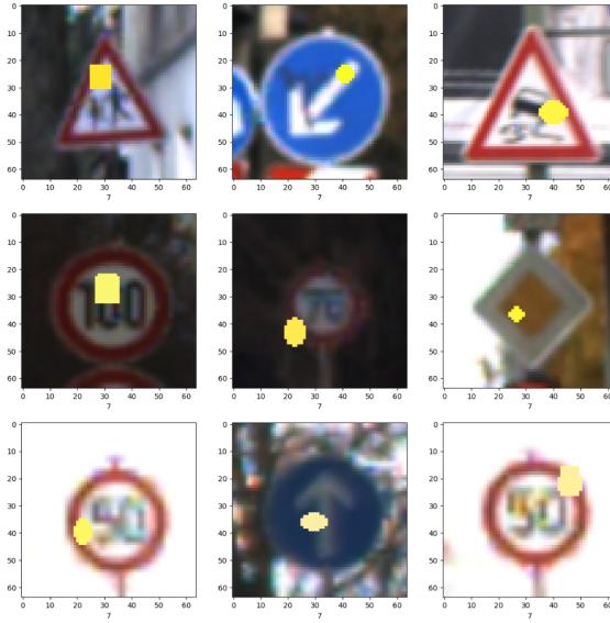
Figure 6: Variable trigger added to downscaled images. The trigger changes in position, shade, and size, so the model is able to later associate a similar physical trigger with this artificial trigger.
