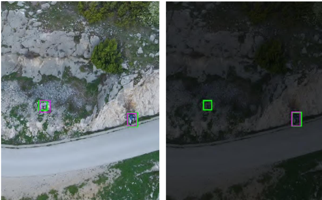
(a) Image from HERIDAL dataset with correct human detection (b) Darkened and noisy version of the same image: the person on the left is not detected
