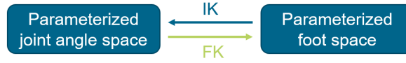
Figure 2.2: Relationship between active joint angle space and foot space. The feasibility assessment is simpler when creating the trajectories in the parameterized foot space.
