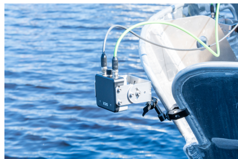
Fig. 1. 1D FMCW radar sensor mounted at the bow of our research boat.
