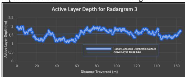
Fig. 4: Depth to Active Layer Reflector of Radargram 3 determined assuming a constant velocity of .1 m/ns.
