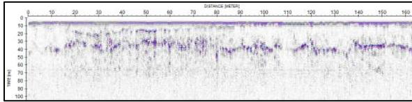
Fig. 3: Radargram 3 processed with 100 and 800 MHz filters and Topographic Correction.
