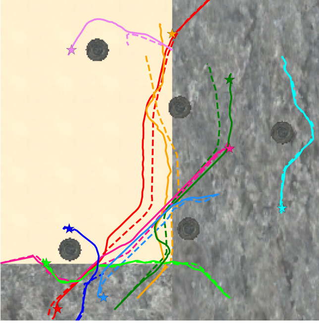
Fig. 8: The trajectories of the robot for both full-body (solid lines) and body-only (dashed lines) planning are illustrated as they navigate a feature-light environment towards designated goals (stars). Lines of the same color are associated to the same start and goal conditions.
