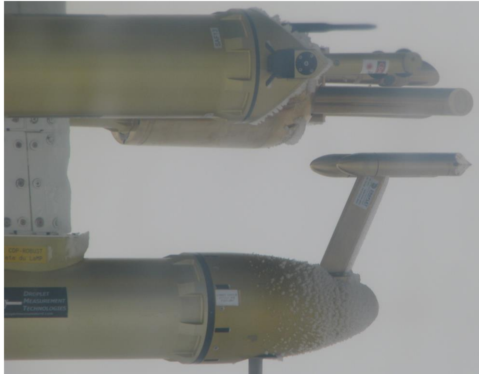
Reference sensors with ice accretion [image DLR with Safire permission]
