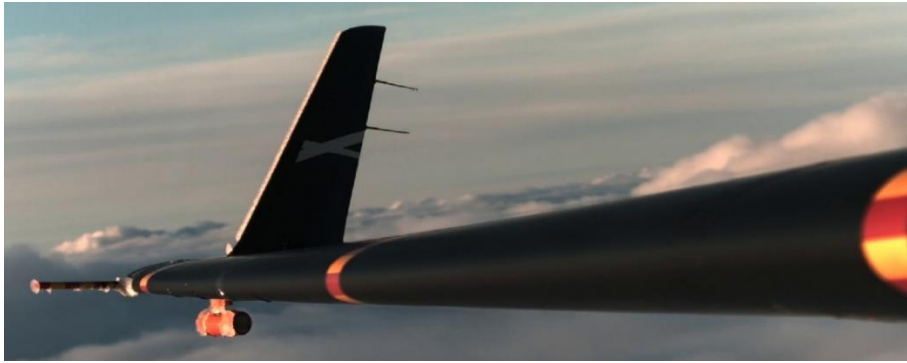
Figure 6 Embraer Phenom 300 with ice accretion on wing tip [copyright Embraer]
