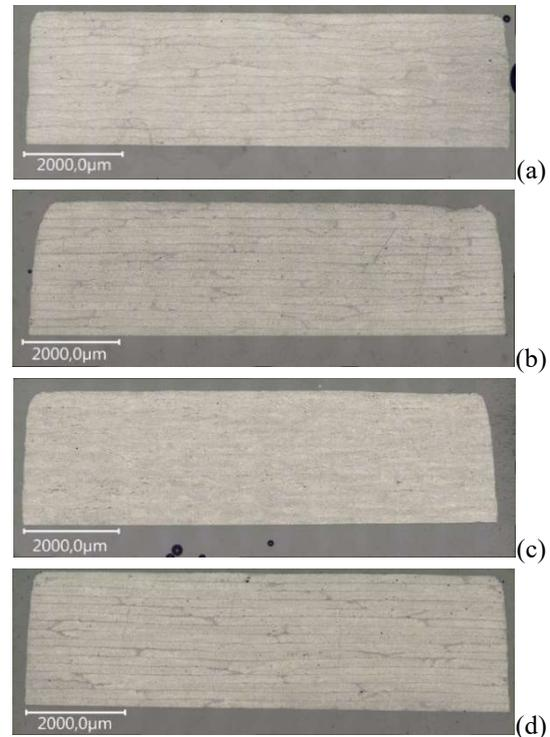
Fig. 2: Microsections from different samples Benchmark (a), Suprem 55 % in-situ (b), Toray 60 % in-situ (c) and Suprem 55 % annealed at 200 °C (d)
