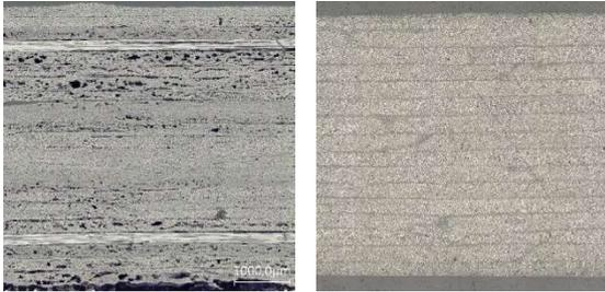
**Fig. 1:** Comparison of microsections taken from the MFFD window cutout (left) and the lab specimen placed in-situ with Suprem 55% LM-PAEK (right)
