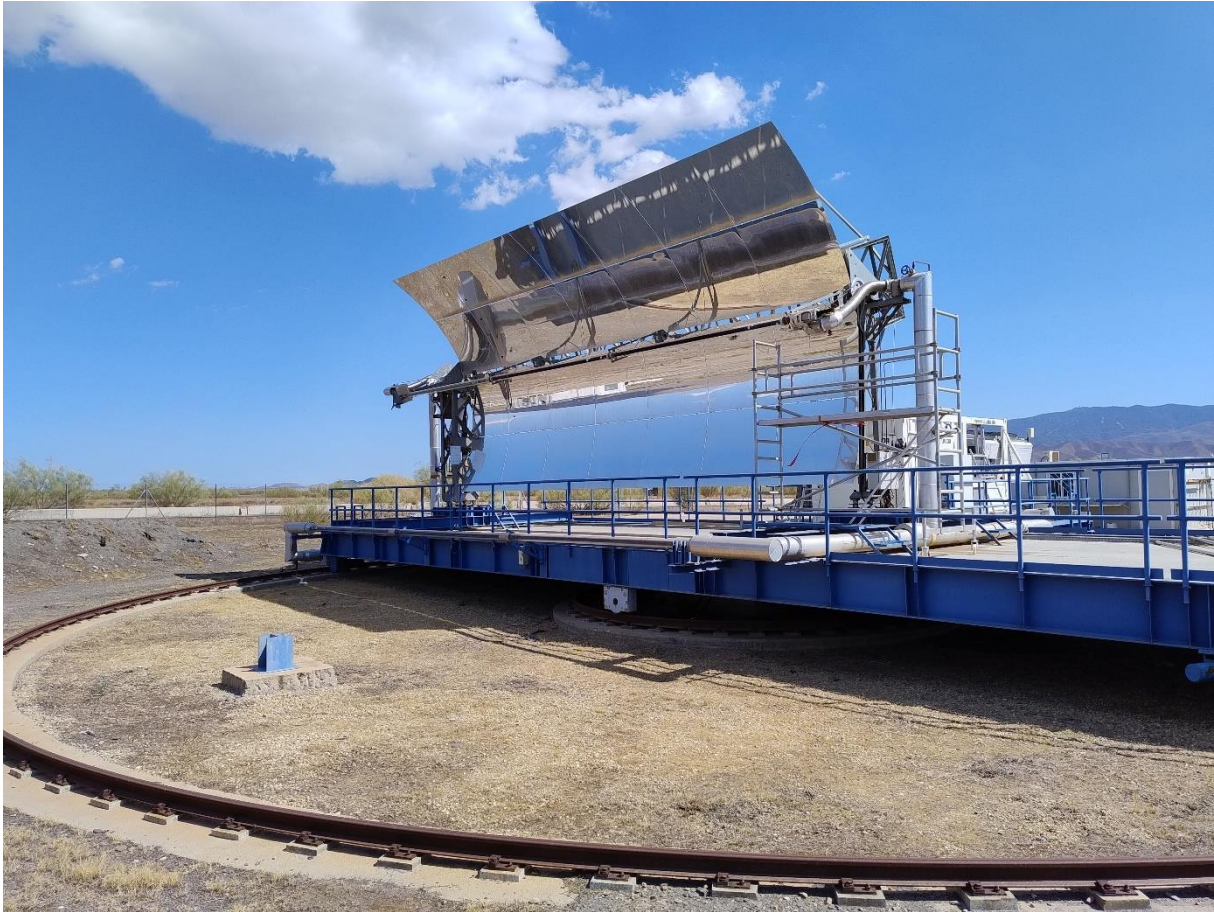
Figure 8 KONTAS test bench with its rotatable platform
