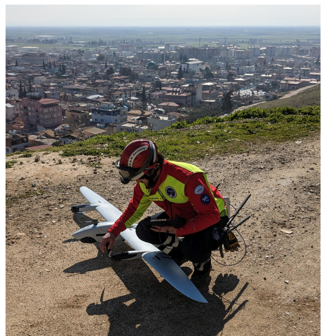
Figure 1. VTOL drone with aerial camera ready for survey flight
