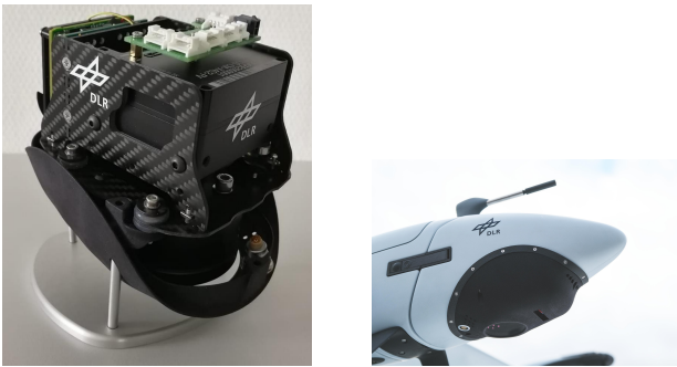
Figure 2. MACS-nano aerial camera (left) and integrated in VTOL fixed wing drone (right)
