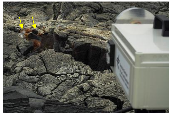
Fig.1-VEMulator2.0 targeting fumarolic deposit and alteration products due to escaping hot gases from a fracture - the 2022 lava field of Fagradalsfjall. Calibration targets (black rectangle (8cm in length) and gray circle) are shown with yellow arrows.
