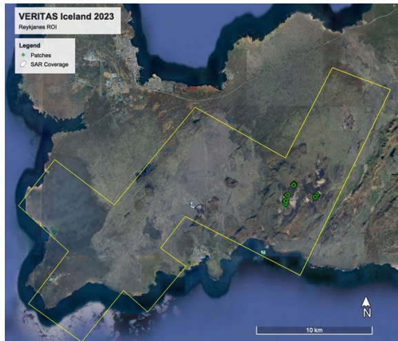
Fig. 3 – F-SAR coverage (yellow polygon) and location of surface characterization patches (green markers) in the Reykjanes ROI. Note that the surface effort concentrated on the 2021-2023 Fagradalsfjall volcanic flows (Background image: Google Earth).
