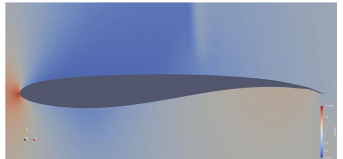
Fig 3: Optimized shape with diffusion constraint. Cl = 0.50 , t = 0.105 , Cd = 0.038
