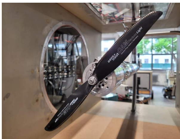
Figure 1: Test section. Rotor with glued dots on blades used to study the effects of boundary layer transition on vortex pairing
