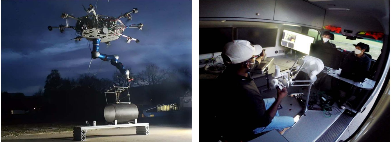
Figure 1: Left: the cable-Suspended Aerial Manipulator, dubbed SAM [1] during field experiment. Right: a ground station where an operator remotely controls the robotic arm through a haptic interface. In real-world applications of bilateral teleoperation, the operator is often remotely located without visual contact to the robot.
