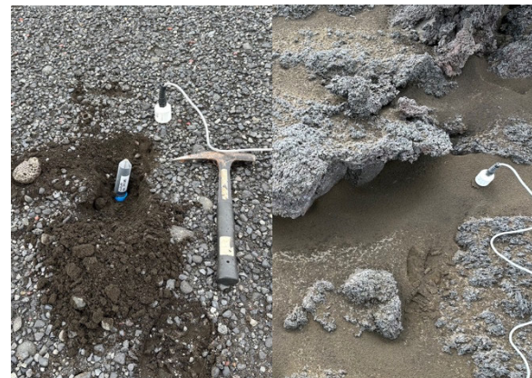
Fig. 2 – (Left) Probing and sediment sampling at a patch on Dyngjusandur. (Right) Probing on sediments collecting on top of the Holuhraun flow. Diameter of probe head (white cylinder with wire) is 42 mm.
