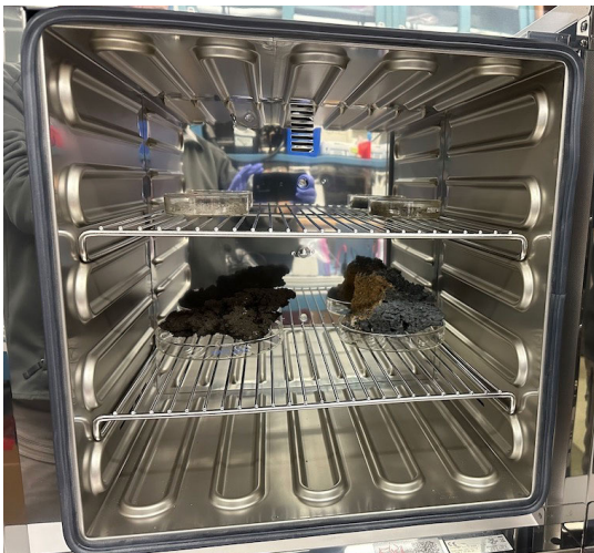
Fig. 4 – Fines (top rack) and rocks (lower rack) resting in petri dishes and within a convection-driven oven ready for drying at 50°C.
