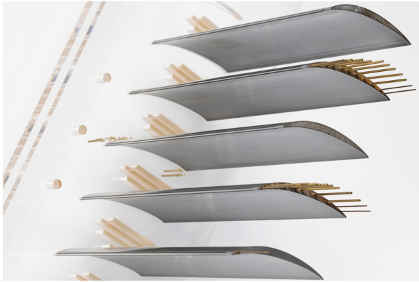
Fig.1 DLR Low Reynolds Number Cascade
