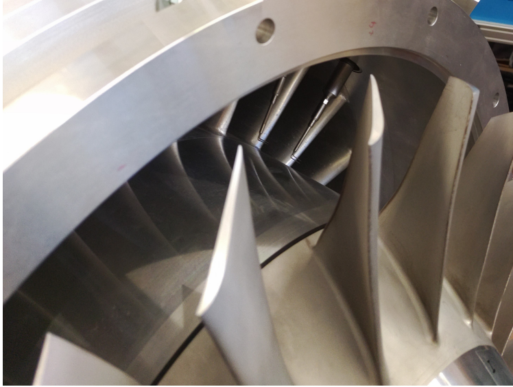
Figure 4 Photograph of two hot wire probes, mounted downstream of the rotor
