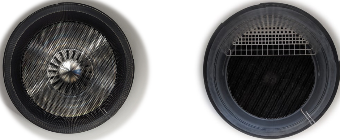
Figure 3 Tested inlet configurations: (left) flow straightener as clean configuration; (right) distortion fence designed for reproduction of a realistic BLI profile
