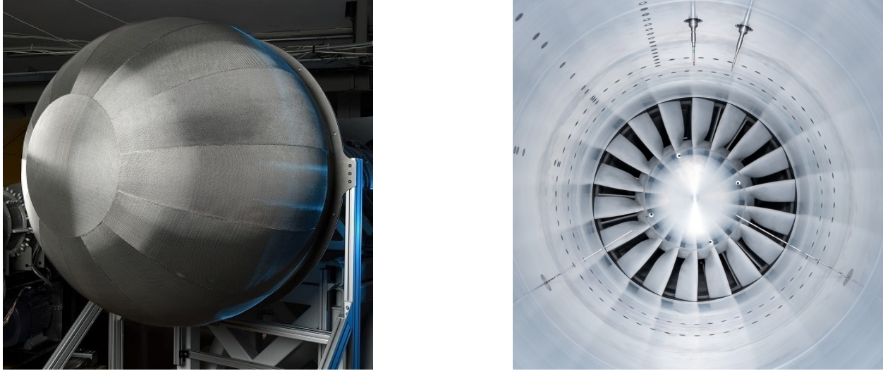
Figure 2 (left) inflow control device; (right) front view of the fan with aerodynamic measurement probes installed
