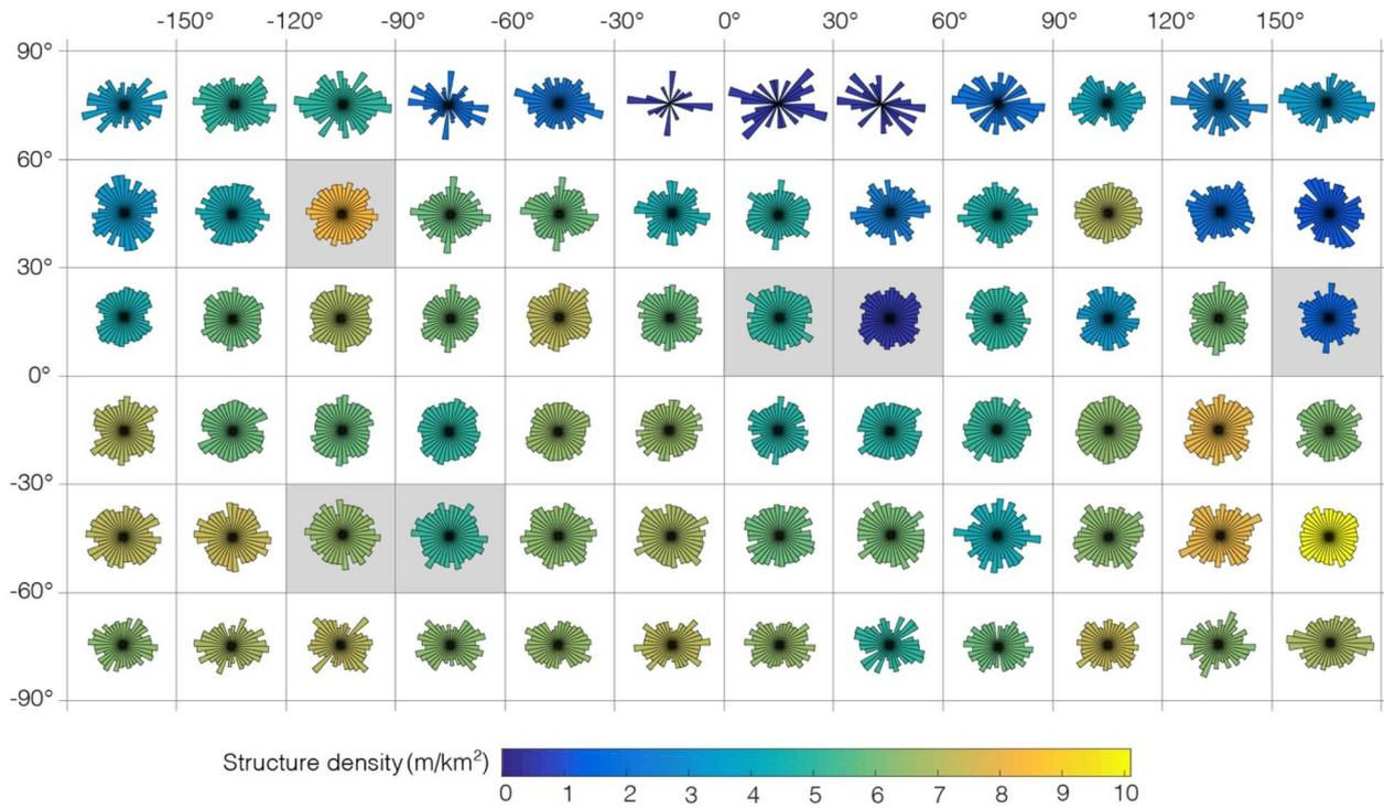
**Figure 5.** Orientations of straight rim segments on Mercury shown as rose diagrams arranged in equirectangular projection. Density of measurements per bin is color coded with warmer colors representing higher densities and cooler colors representing lower densities. Rose diagrams with orientation distributions indistinguishable from uniform are shown with gray background and those with non-uniform distributions have a white background.
