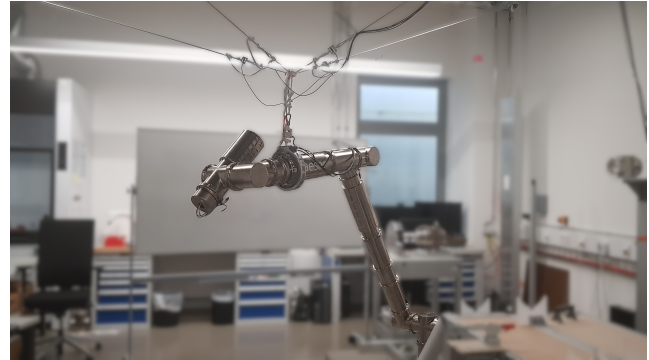
Fig. 1. CAESAR robotic arm, supported by a Motion Suspension System, Credits [3], Copyright © 2023, IEEE
