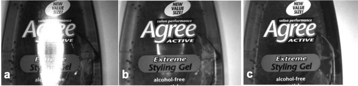
Figure 2.7: Specular vs Diffuse Lighting example from [68]: a. Ring Light without Polarizers, b. Ring Light with Polarizers c. Ring Light with Polarizers and in Diffuse mode. a. and b. are captured in bright field forward mode. a. produces strong reflection due to the illumination mode and the lack of polarizer. b. produces little glare even with polarizer, which filters out some of the reflections. c. produces no reflections due the combination of Diffuse Lighting mode and Polarizers.
